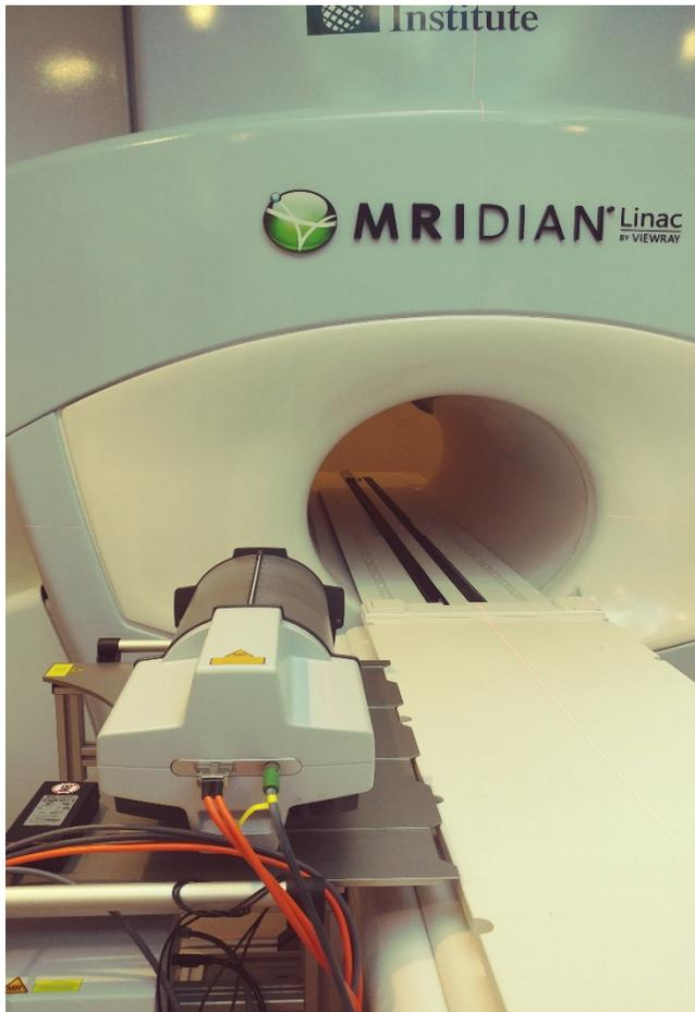
Figure 1. Delta<sup>4</sup> Phantom+ MR. A portable table is included for transportation and easy placement onto the LINAC couch.
