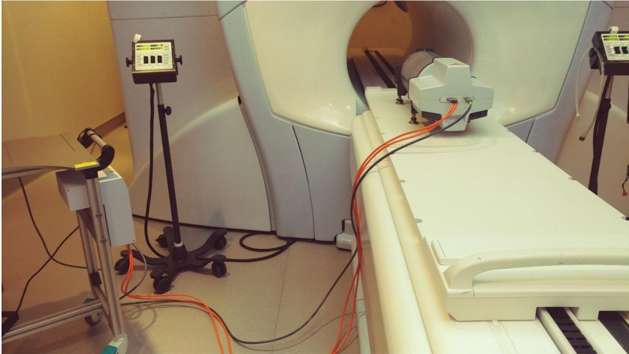
Figure 2. Delta<sup>4</sup> system setup for measurement
